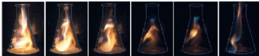
Figure 2: Ignition in an Erlenmeyer flask during determination of ignition temperature
