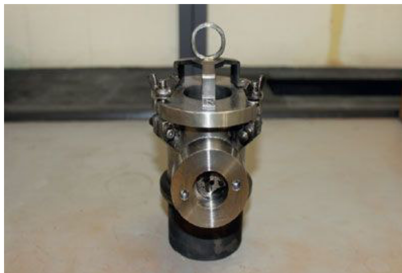
Figure 6: Pressure vessel used in the Dutch pressure vessel test
